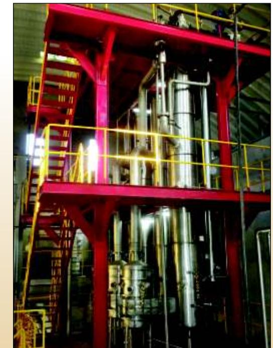
Falling film evaporators are highly responsive to alterations of parameters such as energy supply, vacuum, feed rate, concentrations, etc. When equipped with a well designed automatic control system they can produce a very consistent concentrated product.
